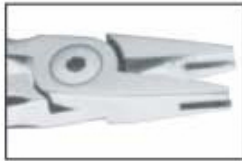
45.9063.13 "V" bend stop special design makes 1mm "v" bends to shorten archwires or provide a positive stop. Excellent for placing stops in titanium wires. For round or rectangular wires up to .025"
